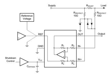
Figure 6. SGM8199 Transient Protection Using a Single Transzorb and Input Clamps
