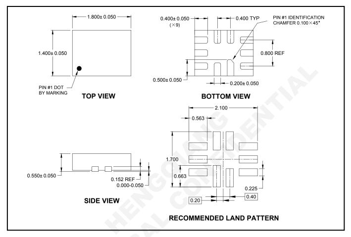
NOTE: All linear dimensions are in millimeters.
