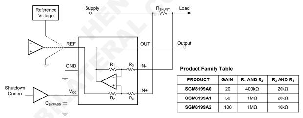
Note:  $400k\Omega$  or  $1M\Omega$  pathes from shunt inputs to reference and SGM8199 outputs.
