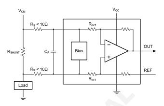
Figure 2. Filter at Input Pins
