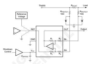
Figure 5. SGM8199 Transient Protection Using Dual Zener Diodes
