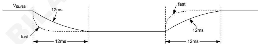
Figure 3. V ELVSS Transition Time Control
