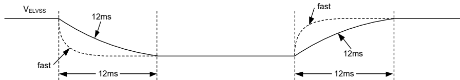
Figure 3. V_{ELVSS} Transition Time Control
