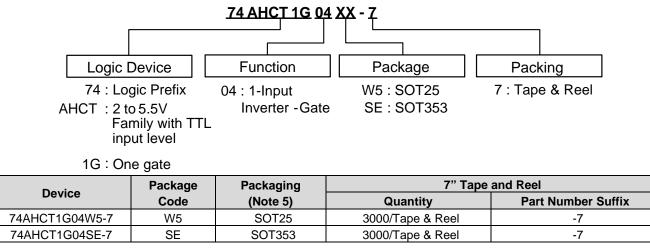
Notes: 5. Pad layout as shown on Diodes Inc. suggested pad layout document AP02001, which can be found on our website at http://www.diodes.com/datasheets/ap02001.pdf.
