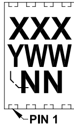
8-Lead DFN (3x3x0.9 mm) (MCP662)
