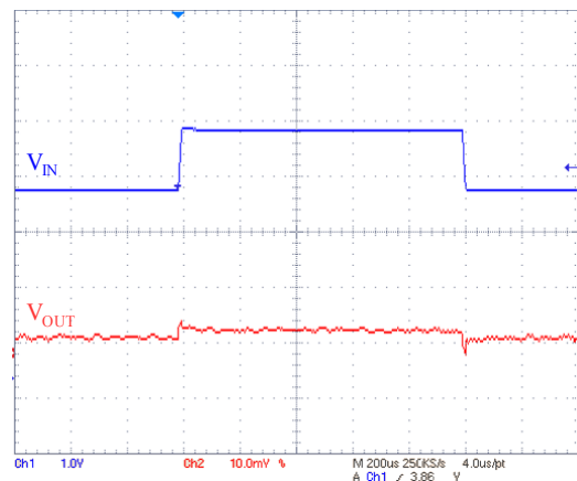
Figure 25. Line transient ( I_{OUT} = 250\text{ mA} )
