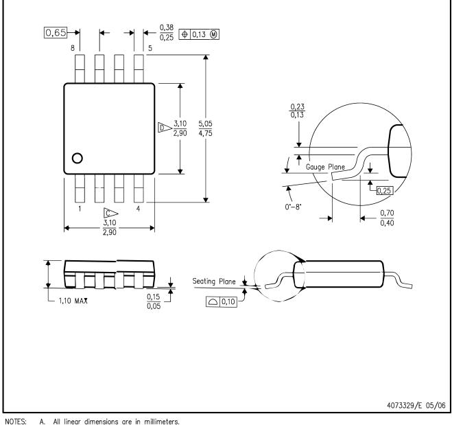
Α. All linear dimensions are in millimeters.
