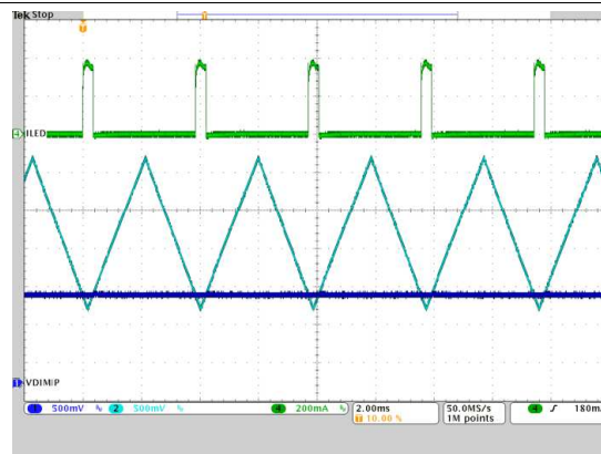
Ch1: Dim/PWM voltage; Ch2: RAMP pin voltage; Ch4: LED current; Time: 2 ms/div Figure 47. Analog-to-PWM Dimming Transient
