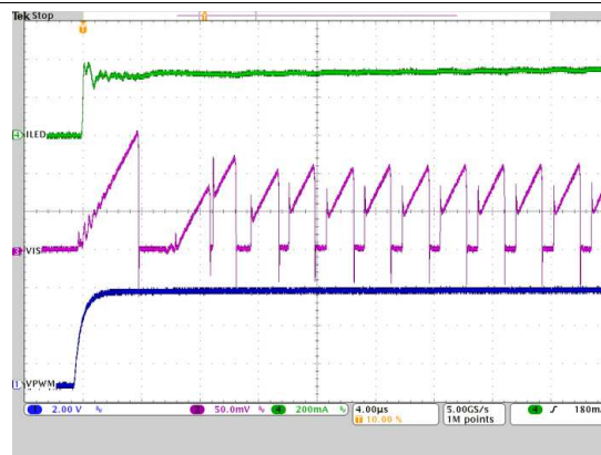
Ch1: External PWM input voltage; Ch3: Switch sense current resistor voltage; Ch4: LED current; Time: 4 \mu s/div Figure 49. PWM Dimming Transient (Zoomed)
