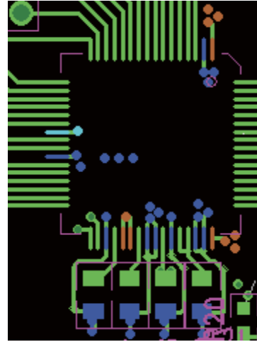
图62. REFIN/REFOUT、REFCAPA、REFCAPB和REGCAP引脚的顶层去耦
