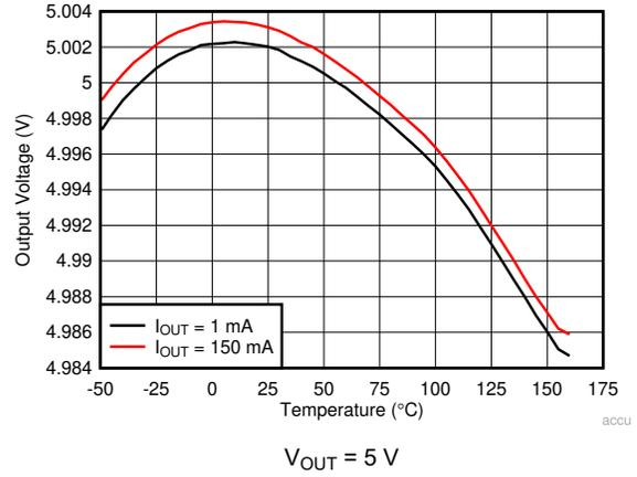
Figure 6-8. Output Voltage vs Ambient Temperature
