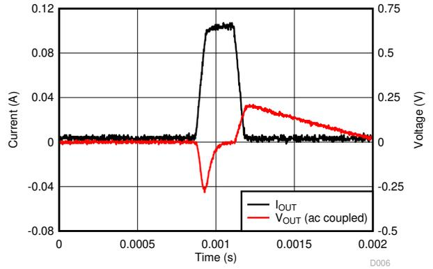
Figure 6-20. Load Transient
