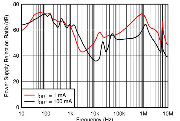
Figure 6-22. PSRR vs Frequency
