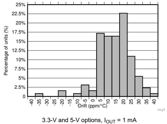
Figure 6-10. Temperature Drift Histogram (-40°C to +25°C)
