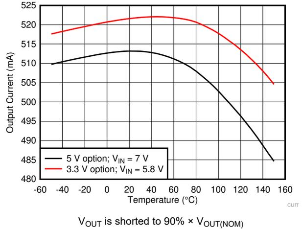
Figure 6-14. Output Current Limit vs Ambient Temperature
