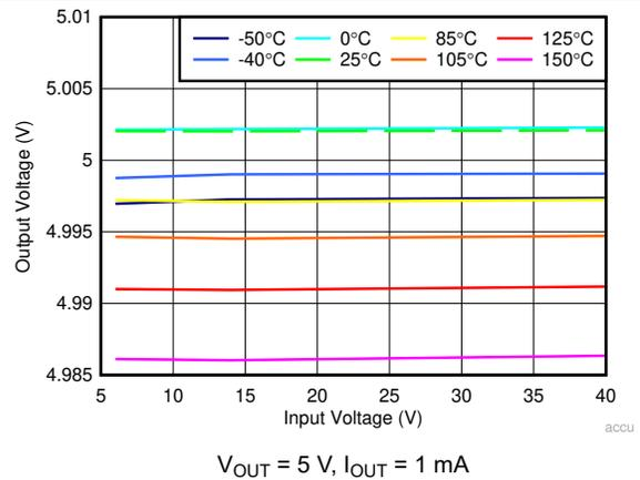
Figure 6-12. Output Voltage vs Input Voltage
