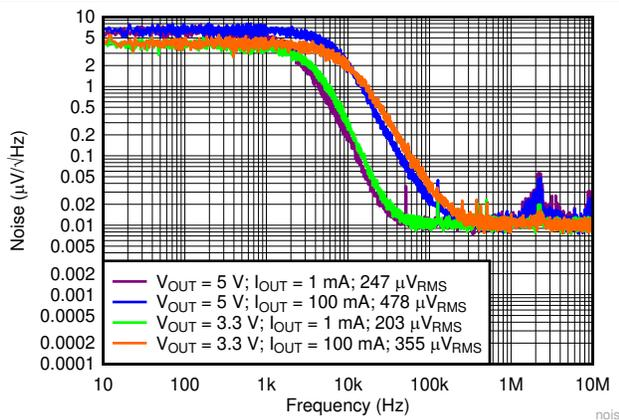
Figure 6-23. Noise vs Frequency
