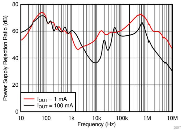
Figure 6-21. PSRR vs Frequency
