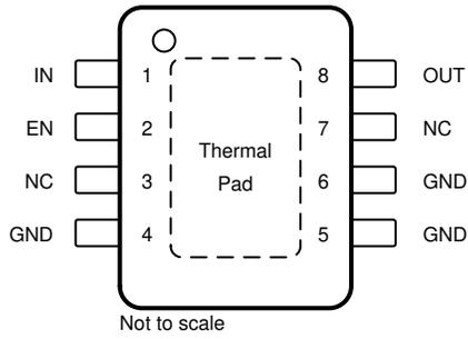
Figure 5-1. DGN Package, 8-Pin HVSSOP PowerPAD™, Top View
