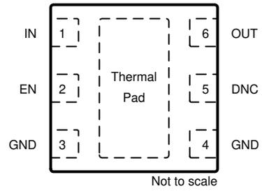
Figure 5-2. DRV Package, 6-Pin WSON PowerPAD™, Top View
