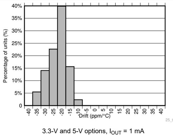
Figure 6-11. Temperature Drift Histogram (25°C to 150°C)
