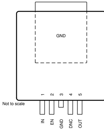
Figure 5-3. KVU Package, 5-Pin TO-252, Top View
