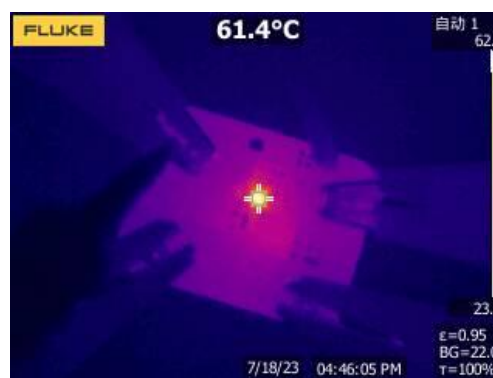
Figure 20. Thermal, VIN=5V, VOUT=1.2V, ILOAD=3A
