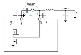
Figure 6. Snubber circuit
