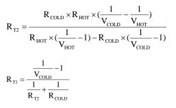
Where,  $R_{HOT}$  is the NTC resistance at the hot temperature threshold,  $R_{COLD}$  is the resistance at the cold threshold.
