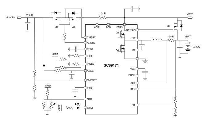
Figure 1. SC89171 with powerpath application
