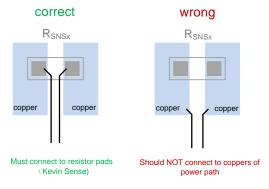
Figure 7. Current sense circuit
