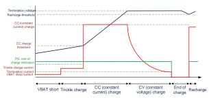
Figure 3. Typical charge profile
