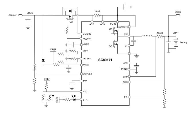
Figure 2. SC89171 without power path application
