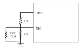
Figure 5. NTC Circuit
