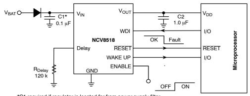
\*C1 required if regulator is located far from power supply filter.
