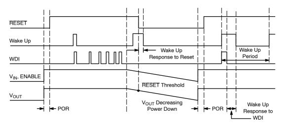
Figure 4. Power Down, Restart Sequence, and Wake Up Response to WDI
