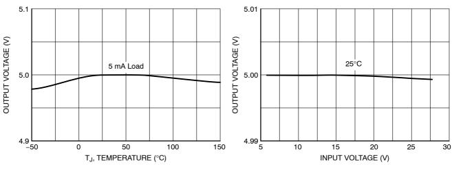
Figure 5. Output Voltage vs. Temperature
