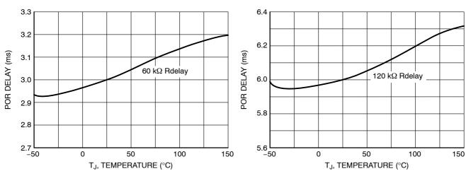
Figure 7. POR Delay vs. Temperature, 60 k $\Omega$  Rdelay
