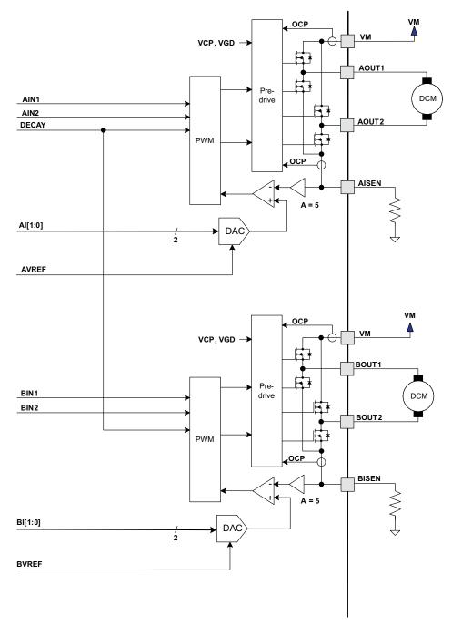
Figure 5. Motor Control Circuitry
