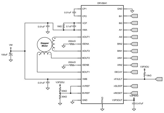
Figure 7. Typical Application Schematic
