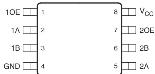
Figure 5-2. DCU Package 8-Pin VSSOP Top View
